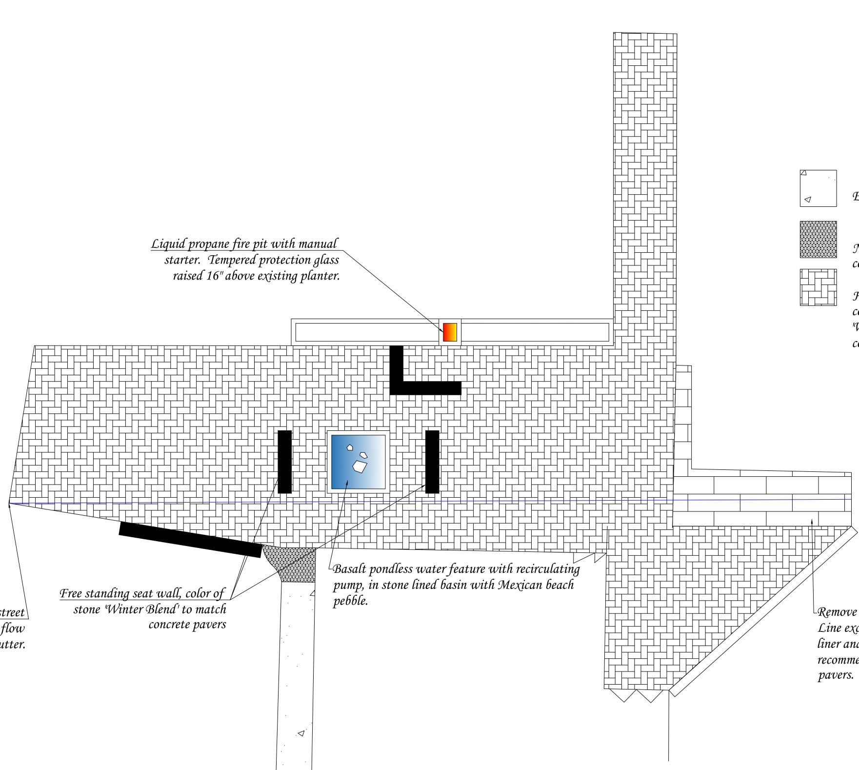
Extend drainage pipe 66LF to street ensure 1% fall. Drain pipe into flow line. Replace sidewalk and curb/gutter.
